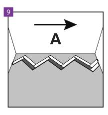
It is very important that the installation of each row is done according to the principle that panels A are installed in the right direction.
