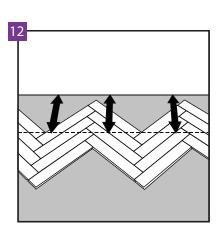
After laying four full rows of panels. Set the line along which the floor will be cut so that the resulting fragment can be moved towards the wall.
