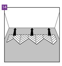
The cut floor should be pushed to the wall with the expansion joint in mind.
