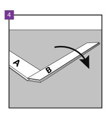
Mount (jam) without driving panel B in with the movement indicated in the figure above.
