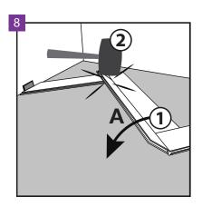
Laying of the second row should also be started with panel A. Please keep the rules in mind at all times concerning installation of the panels – when driving panel B in to panel A, the long sides are installed by jamming, while the short sides are assembled by driving in.
