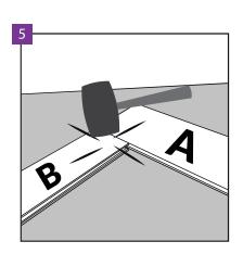
Then put panel A. Then connect panel B to panel A using a rubberized hammer. Note! Each panel contains only 1 lock that can be pinned down. Other locks must be installed without driving in (see installation, Figure 4). Note! Try the lock very carefully before driving in (lack of precise fit of the lock and then driving the panel in will cause its damage, which will result in rejecting a possible claim).
