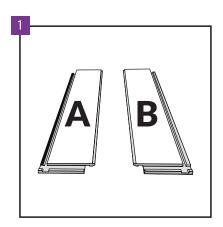
Each package contains two types of panels: A and B. The individual panels are marked at the bottom as A or B for easier differentiation. Parts A and B must be sorted separately before the installation. During installation, it is very important to ensure that panels A and B are installed at the right places in the row (see -> panels laying, point 7; 9 and 10).
