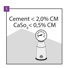
In the case of the cement grout, the moisture content in the substrate must be lower than 2.0%, and in the case of the anhydrite grout, it must be lower than 0.5%. In the case of installation with the underfloor heating, the abovementioned values must be 1.5% and 0.3% respectively.
