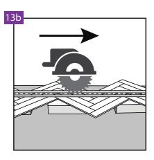
When cutting, we recommend using spacers that must be placed under the floor to avoid damaging the underlay. The height of the spacers should be adjusted according to the guidelines specified by the manufacturer of the circular saw or guide saw.
