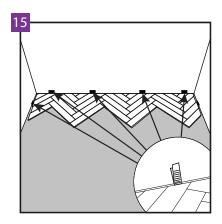
Leave 5 mm of perimeter space at the walls to allow the floor expansion. The maximum surface which can be laid without additional expansion joints is 200 m². Above this surface, apply an additional expansion joint and enlarge all the expansion joints up to 10 mm. The maximum length of the floor surface in one direction, which can be laid without additional expansion joints is 20 m. Above this length, apply an additional expansion joint and enlarge all the expansion joints up to 10 mm.
