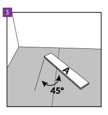
Start the installation from left to right from panel A, which should be rotated at 45°. The edge panels along the wall should be cut to size at 45° matching the walls. NOTE! Taking care to keep the appropriate wall expansion joints (see installation, Figure 15).
