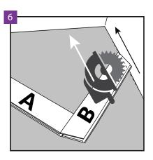
Install next B panel in the same row (see floor installation manual – Fig. 4). Cut the panel making sure to use proper wall expansion joints (see floor installation manual – Fig. 15).
