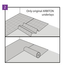
Make sure that the substrate is properly prepared. Then lay the Arbiton or Ewifoam brand underlay, which is designed for installation of rigid and LVT floors. The neighbouring ribbons of underlay must fit tightly and must be joined by means of an overlap or Arbiton or Ewifoam AluTape, without leaving any redundant space.
