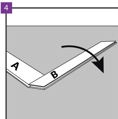
Mount (jam) without driving panel B in with the movement indicated in the figure above.
