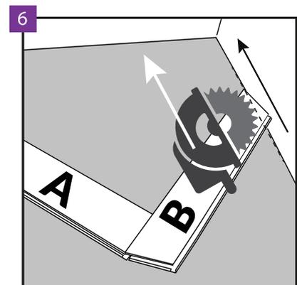
Install next B panel in the same row (see floor installation manual – Fig. 4). Cut the panel making sure to use proper wall expansion joints (see floor installation manual – Fig. 15).
