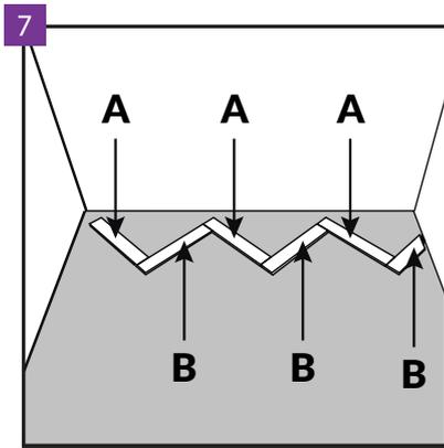
The first row should consist of alternately arranged panels, which will be mounted in exactly the same way as in the presented figure.
