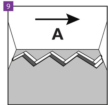
It is very important that the installation of each row is done according to the principle that panels A are installed in the right direction.
