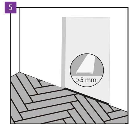
The application of the 5 mm expansion joint in the door opening between the rooms, which allows for the elimination of stresses, is recommended in the following cases: the irregular shape of the floor surface in the neighbouring rooms, the placement of heavy furniture in one of the rooms or the application of the underfloor heating only in one of the joined rooms. In the case of an area bigger than 200 m<sup>2</sup> or longer than 20 m, the expansion joint must be enlarged to 10 mm.
