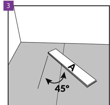
Start the installation from left to right from panel A, which should be rotated at 45°. The edge panels along the wall should be cut to size at 45° matching the walls. NOTE! Taking care to keep the appropriate wall expansion joints (see installation, Figure 15).
