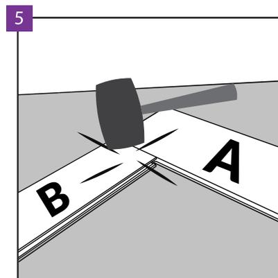
Then put panel A. Then connect panel B to panel A using a rubberized hammer. Note! Each panel contains only 1 lock that can be pinned down. Other locks must be installed without driving in (see installation, Figure 4). Note! Try the lock very carefully before driving in (lack of precise fit of the lock and then driving the panel in will cause its damage, which will result in rejecting a possible claim).
