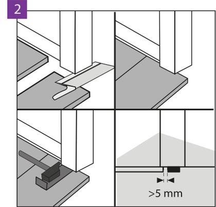
At the doors, it is recommended to undercut the profiles of door frames and leave free space over the installed panel so as not to limit its possible movement.
