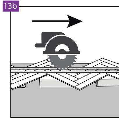
When cutting, we recommend using spacers that must be placed under the floor to avoid damaging the underlay. The height of the spacers should be adjusted according to the guidelines specified by the manufacturer of the circular saw or guide saw.
