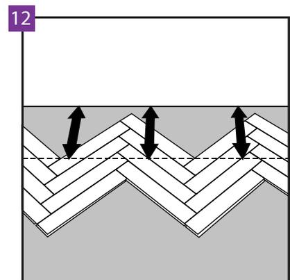
After laying four full rows of panels. Set the line along which the floor will be cut so that the resulting fragment can be moved towards the wall.
