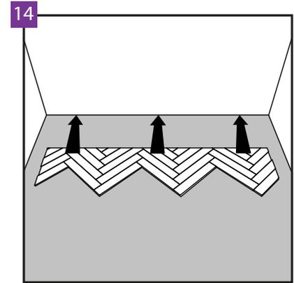
The cut floor should be pushed to the wall with the expansion joint in mind.
