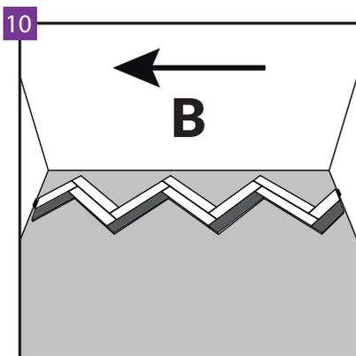
It is important that the assembly of each row is carried out with the principle that we assemble panels B to the left, i.e. the opposite direction of the assembly of panels A.
