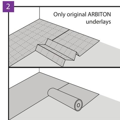
Make sure that the substrate is properly prepared. Then lay the Arbiton or Ewifoam brand underlay, which is designed for installation of rigid and LVT floors. The neighbouring ribbons of underlay must fit tightly and must be joined by means of an overlap or Arbiton or Ewifoam AluTape, without leaving any redundant space.
