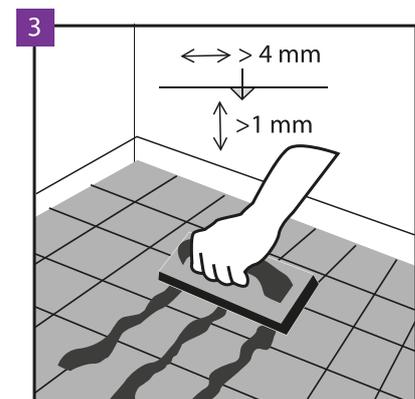
In the case of installation on the substrate covered with ceramic tiles, fill the tile joints with the gap wider than 4 mm and deeper than 1 mm with a durable compound for the filling of points, e.g. resin grout. Installation is allowed on tiles with grouts not wider than 5 mm and 1 mm deep without using levelling compound, provided the Arbiton or Ewifoam brand underlay, which is designed for installation of rigid and LVT floors.
