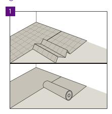
Lay the Arbiton, Ewifoam or Afirmax underlay perpendicularly to the direction in which panels are laid. The neighbouring ribbons of underlay must be fit tightly and joined by means of an overlap or Arbiton AluTape, without leaving any redundant space.
