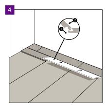
The Arbiton floor panels are provided with locks on the short and long side. First, connect the panel on the long side; for this purpose slide the long side of the panel into the groove of the previously installed row of panels. Move to the corner, leaving some clearance.
