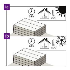
If the temperature is >5°C during transport, the acclimatization time in a room with a temperature of 18-30°C should be min. 24 hours (in the premises where they will be installed). However, in case of temperature ≤5°C during transport, acclimatization time in a room with a temperature of 18-30°C should be min. 48 hours.
