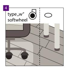
Used office chairs with W-type castors, protecting the floor additionally by means of the protective net. The furniture legs must be provided with protective pads which provide protection against scratching, e.g. made of felt.
